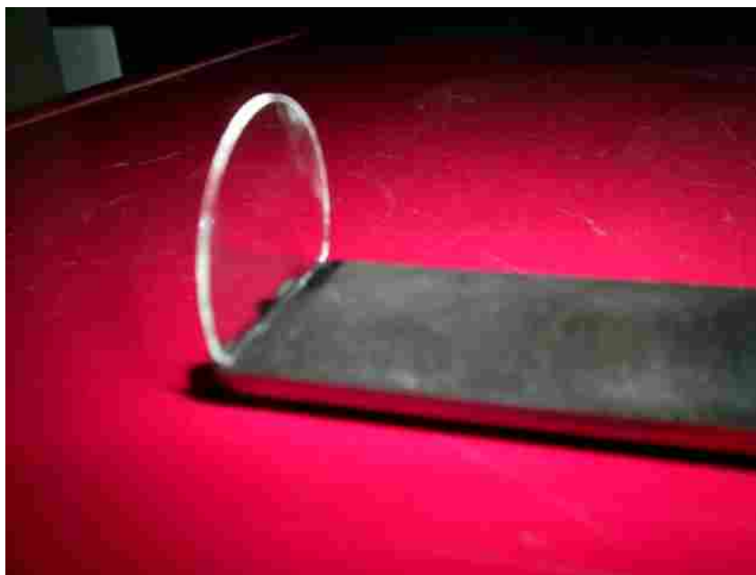
Figure 3-15 Sample holder with bare glass sample installed
